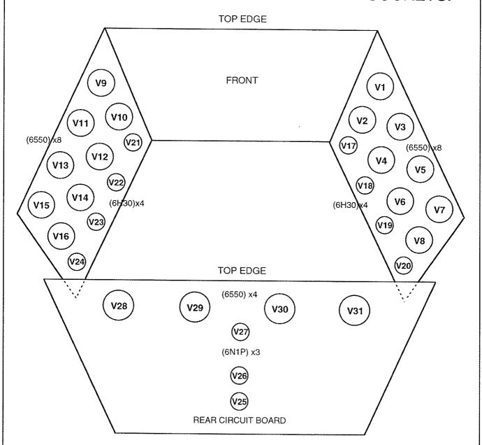
RELATIVE POSITIONS OF ALL (31) TUBES LOCATED ON THREE CIRCUIT BOARDS AS VIEWED FROM THE REAR AND LOOKING DOWN FROM ABOVE THE AMPLIFIER.
